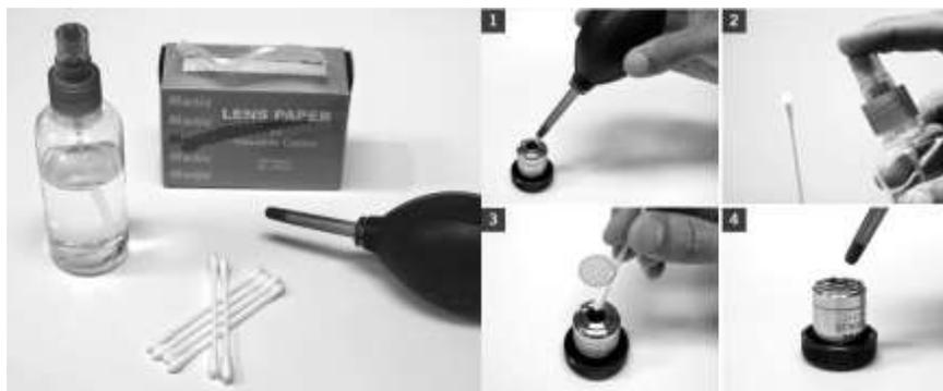
**For objectives that work with immersion oil** it is essential to clean them after each observation session. To clean use a cleaning cloth for lenses slightly dampened with a low graduation of alcohol. Proceed by cleaning
