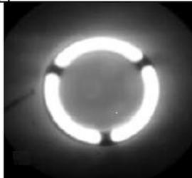
R. Repeat above steps with the 20x, 40x and 100x phase objectives, making sure to position the corresponding annuli of phase turret condenser to matching objective indexed in optical path. (Plan 10Ph/0.25 matched to the number 10 on rotating phase turret condenser.)
