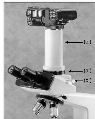
inch chip, remove only the top black knurled ring from c-mount by turning counter-clockwise. The remaining black knurled ring is a "C" type adaptor.
