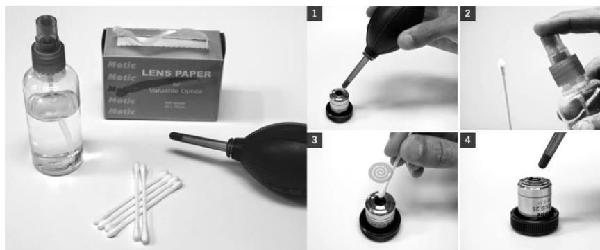
**For objectives that work with immersion oil** it is essential to clean them after each observation session. To clean use a cleaning cloth for lenses slightly dampened with a low graduation of alcohol. Proceed by cleaning the frontal objective lens (normally 100X-Oil). It is important for those objectives that work at a very close distance to the sample.
